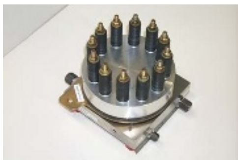
Figure 3. Photograph of the commercial-type PEM electrolyser on the left and the USC research electrolyser installed in the test facility on the right
