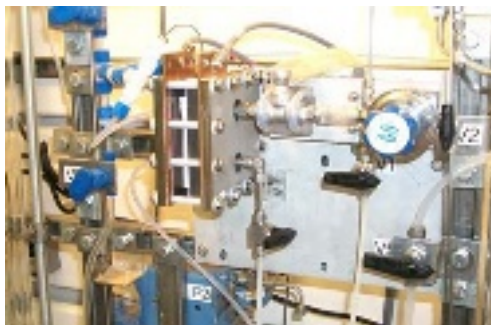
Figure 3. Photograph of the commercial-type PEM electrolyser on the left and the USC research electrolyser installed in the test facility on the right
