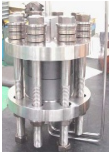
Figure 9. SIC block for seal performance test
